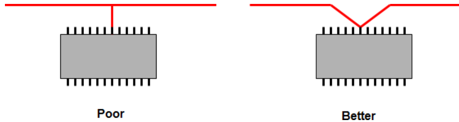
Figure 9. Avoid Right-Angle Traces
