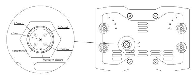
The connector on the WaveSculptor and other Tritium devices is Male, M12, A-coded. The pinout follows the DeviceNET specification, and the diagram above shows the connector on the WaveSculptor as viewed from the front of the controller.
