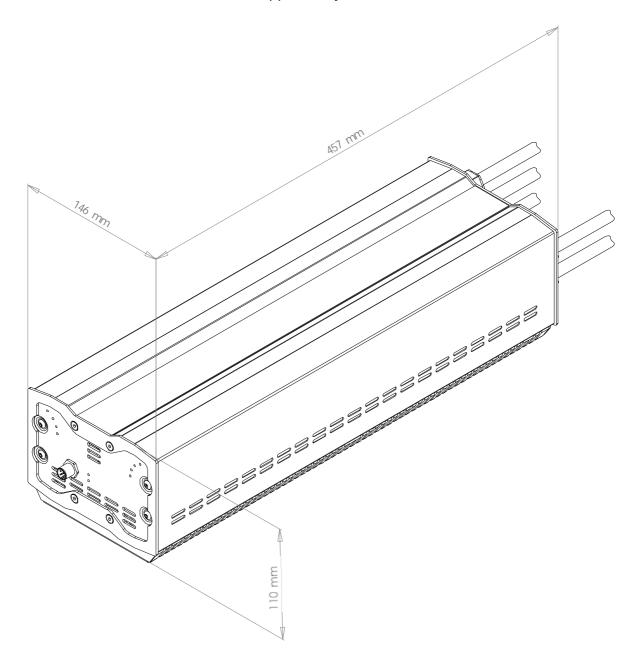
Sufficient room must be allowed at each end of the controller for unobstructed airflow, and to allow clearance for CAN bus, Motor and DC power cabling and connectors.
