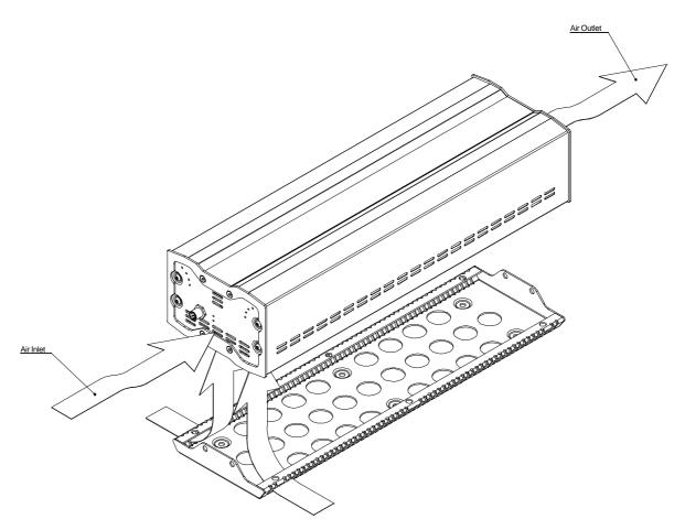
The average power quoted in the controller datasheet is for an ambient temperature of 40°C. Providing air at a lower temperature than this will allow the controller to operate using lower fan speeds (less power consumption), or alternatively, allow operation at higher average power levels.
